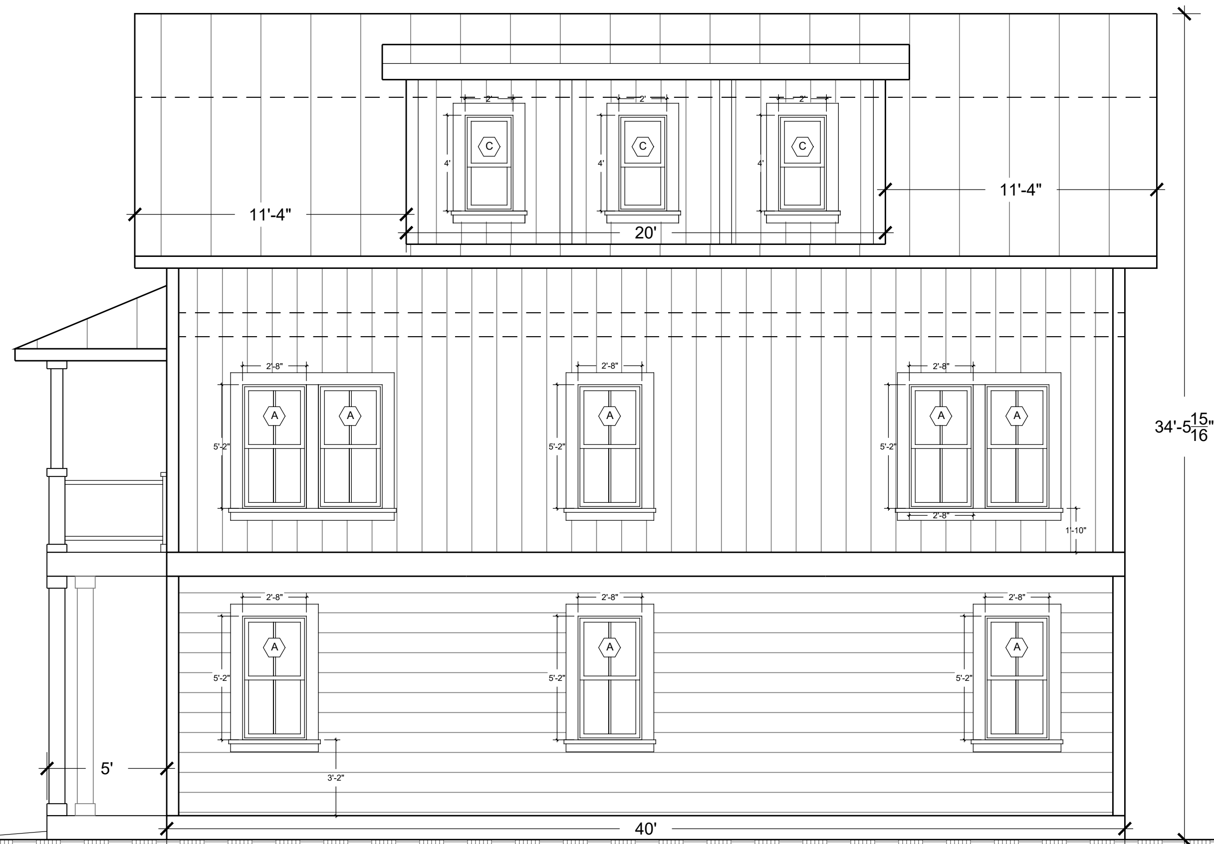
2 UNIT-1 REAR ELEVATION- SOUTH SCALE: 1/4" = 1'-0"
