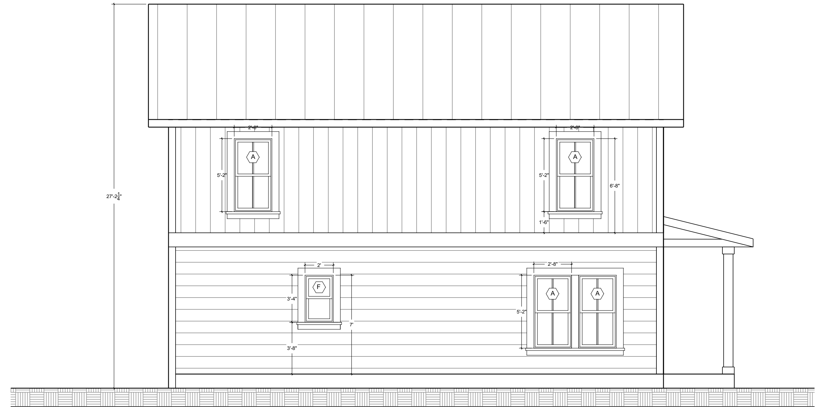
2 UNIT-4 SIDE ELEVATION- NORTH SCALE: 1/4" = 1'-0"
